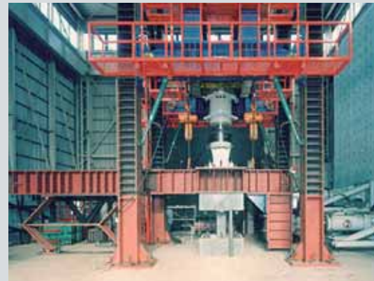
Structural testing of superhigh-strength RC columns
