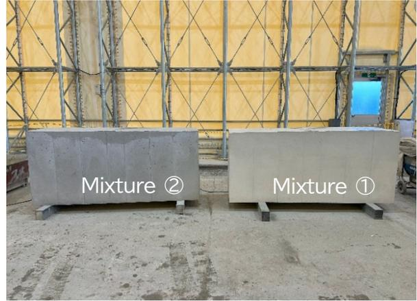
Picture 2: Carbon Negative concrete test specimens
