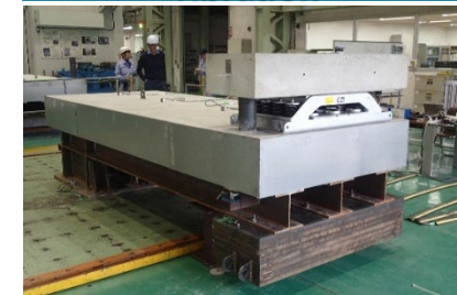
Mass damper for controlling vertical vibration
