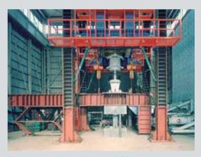
Structural testing of superhigh-strength RC columns
