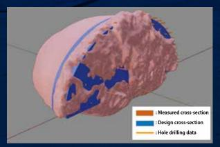
Blasting Design System (Charging and Blasting)
