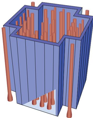
Example of box-shaped diaphragm walls with wide thickness
