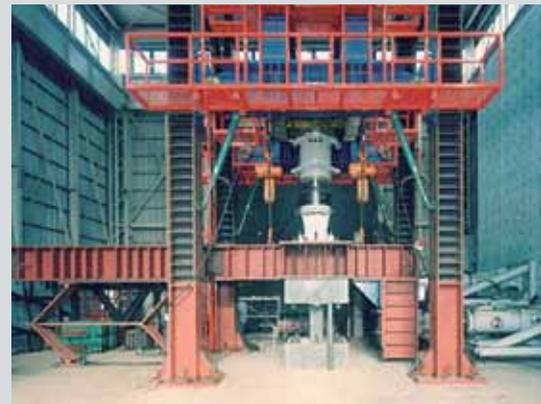
Structural testing of superhigh-strength RC columns
